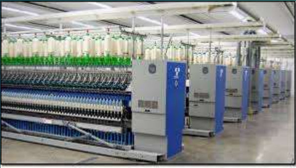
Spinning Unit (183,538 Spindles & 6000 Rotors)
